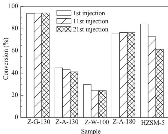
**Fig. 5.** Catalytic cracking conversion of 1,3,5-triisopropylbenzene over different samples after different number of injections. Reaction conditions: 400 °C, 50 mg catalyst, 0.1 μl reactant.
