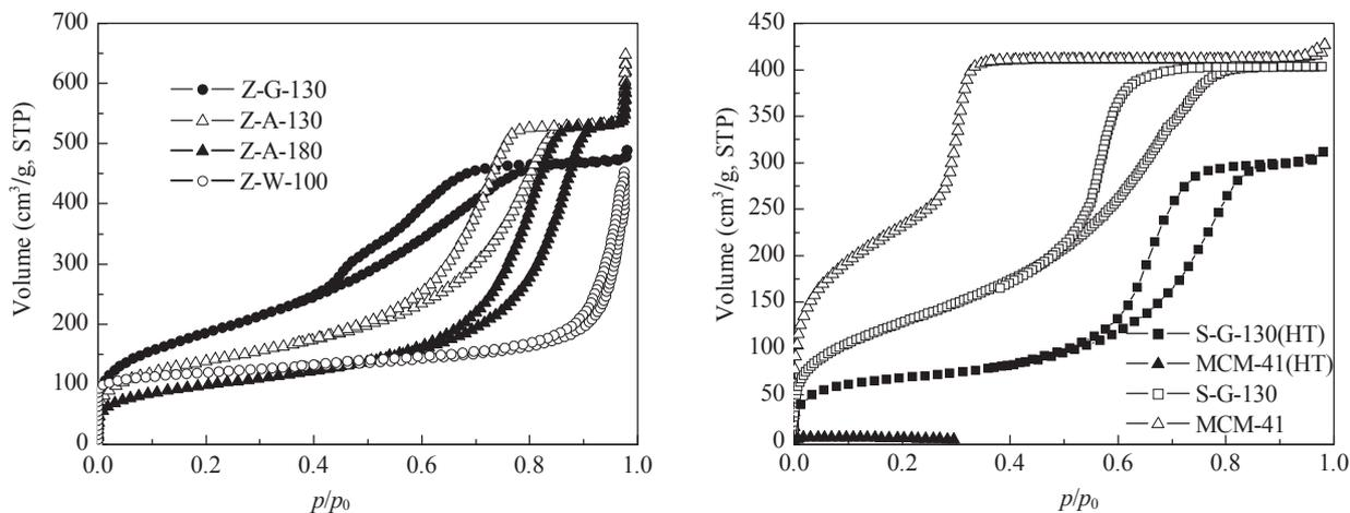
Fig. 3.  $N_2$  adsorption/desorption isotherms of the studied samples. HT represents hydrothermal-treated samples at 180 °C.
