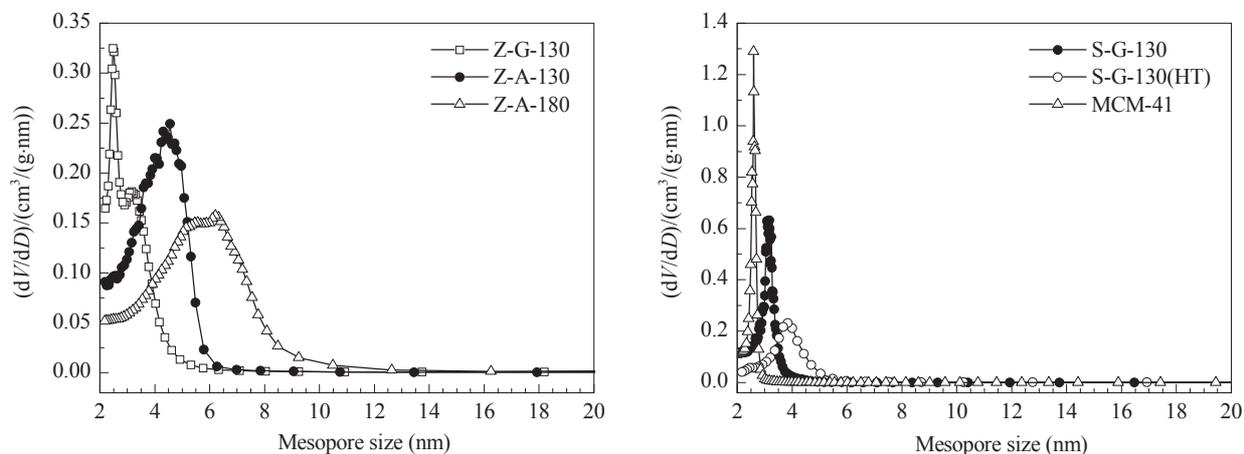
Fig. 4. Mesopore size distributions of the studied samples.
